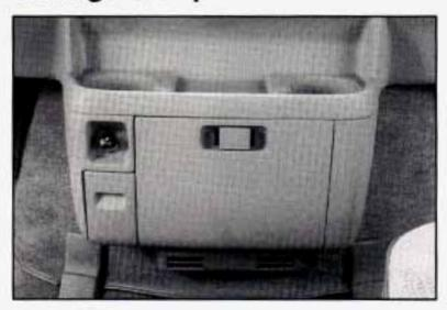
Your front storage compartment is at the center of the engine cover. To open the compartment, press the two tabs together and pull.
